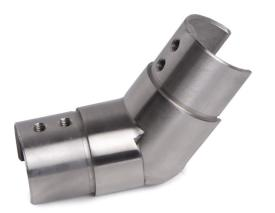
This adjustable elbow for channel tube is made of 316 grade stainless steel and has a brushed finish. It is designed to connect two different ends of 1.67" diameter channel tube, item# A114U and enables an upward bend in the tube. Connect the elbow to the tube ends using our adhesive and activator (items LB-00201 and 00211).
