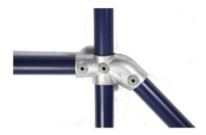
Cross fitting designed for the mid rail on guardrail on slopes and staircases between 30° and 45° at the junction where the handrail changes from either level to sloping down or level to sloping up the stairs.
