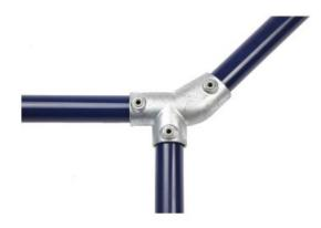
Tee fitting designed for the top rail on guardrail on slopes and staircases between 30° and 45° at the junction where the handrail changes from level to sloping up the stairs.
