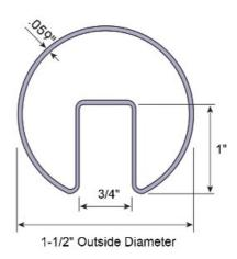
49-A111U architectural round channel tube is available in stainless steel, has a 1-1/2" outside diameter, a 0.059" wall thickness, and is available in stock lengths up to 16 feet.
