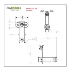
This bracket is designed to mount on to 1.67" diameter vertical posts.
