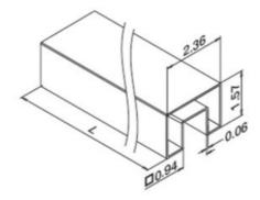
44-6920 architectural rectangular channel tube is available in 304 grade stainless steel, has a width of 2.36", a height of 1.57", and is available in stock lengths up to 16 feet. Finish is satin (brushed).
