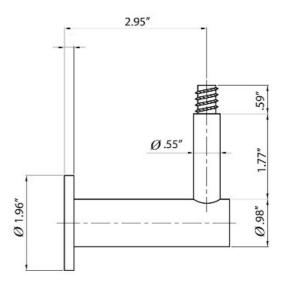
This modern looking handrail bracket is made of 316 grade stainless steel and has a brushed (satin) finish. Use this bracket with A134 wood handrail.
