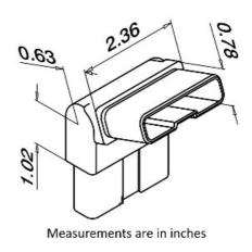
Use this adjustable (articulating) elbow with rectangular tube, item# 49-RL4920/6020.
