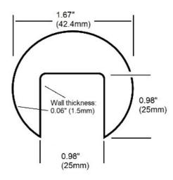
47-A114U architectural round channel tube is available in stainless steel, has a 1.67" outside diameter, a 0.06" wall thickness, and is available in stock lengths up to 16 feet.
