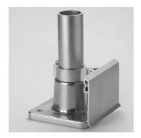
Hollaender's unique beveled toeplate design allows for quick and easy installation. No drilling or welding; an extruded channel allows for secure attachment with no exposed fasteners. Uniform 1/8" wall thickness and beveled shape provides rigid non-buckling performance with the benefit of lightweight, easy handling.
