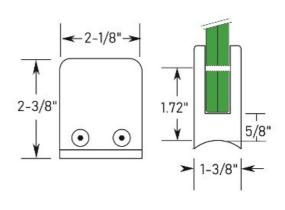
The 44-813/2 square glass grip is made of 304 grade stainless steel, has a satin (brushed) finish, and has a curved back for mounting on 2" OD round tube. It comes with a rubber insert set designed to hold 1/2" thick panels. These glass grips also include a removable pin used to hold the panel in place.
