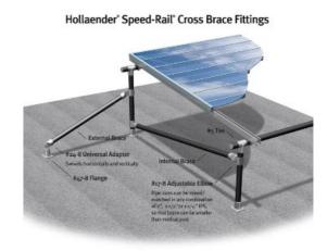
Please note: This fitting is an adapter. One end goes over the 1-1/2" IPS Pipe and the other end goes inside 1-1/2" Fitting.
