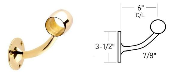
00-520/2 is a wall mount handrail bracket in polished brass and has a ring as a saddle to secure 2" round tube in place. It is ideal for level and stair applications. It can be mounted horizontally at a landing or at the end of a ramp. It can also be mounted at an angle for stair or ramp applications. Each bracket includes two self-drilling screws used to connect to the handrail and three wood screws used for mounting to the wall. Mount the bracket to a stud in the wall.
