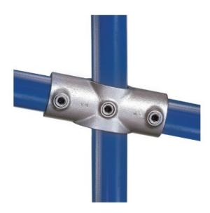
Used to join the middle rail to an intermediate upright on a guardrail on a slope from 0° to 11°. The upright passes through the fitting.
