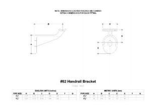
Fits both 1-1/4" and 1-1/2" pipes. Centerline of rail 4-1/8" from wall.
