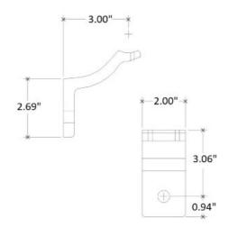
The 07885 handrail bracket is a cast fitting made of aluminum magnesium alloy 535 and is designed to hold 1-1/4" and 1-1/2" IPS pipe.
