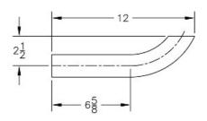
49301L Wall Return Bend LEFT is made of aluminum, is designed to connect to 1-1/2" IPS schedule 40 pipe, and has an anodized finish.
