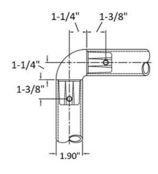
Interna-Rail® item# 58016 is a cast aluminum 90 degree elbow with an anodized finish and is designed to connect with 1-1/2" IPS schedule 40 pipe. This item includes two set screws that are used to connect the pipe to the fitting.
