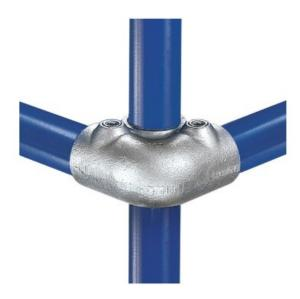
This fitting is designed to provide a 90 degree offset corner joint. When calculating the cutting lengths for pipe, dimension 'G' should be subtracted to give the pipe length for the rails and dimension 'H' should be added to give the pipe length for the upright. To obtain the true height of the upright the allowance for the base fittings must be included.
