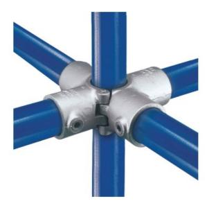
The unique "Hinge and Pin" system of this fitting enables existing structures to be easily extended without the need for dismantling. This fitting is most frequently used in multiple upright structures to tie a center upright with horizontal pipes in four directions. The upright passes through the fitting.
