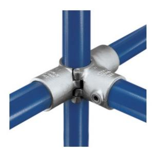
The unique "Hinge and Pin" system of this fitting, enables existing structures to be easily extended without the need for dismantling. This fitting has been designed to tie an upright with horizontal pipes in three directions, all at 90° to the upright. The upright passes through the fitting.
