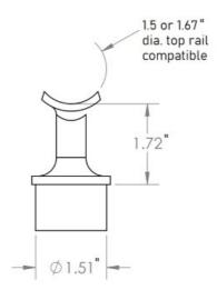
This post mount handrail bracket is made of 316 grade stainless steel and has a brushed (satin) finish. It is designed to hold two tubes of 1.66" diameter tube at 90 degrees. The horizontal tube is fixed in place with two screws and the vertical tube is fixed in place with adhesive see item# LB-00201 and item# 00211.
