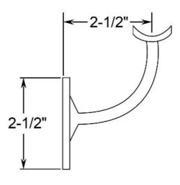
This wall mount handrail bracket is made of 316 stainless steel, has a polished finish and is designed to hold 1-1/2" outside diameter round tube. The back plate has three counter sunk holes that can be positioned for horizontal or angled handrail. Mount this bracket on a wall (recommended on a stud) or on a rectangular vertical post using the included hardware or alternate depending on the material the bracket is being mounted upon.
