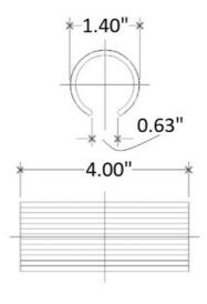
Item 07640 (70E-7) is an aluminum internal coupling (splice) that is designed to connect the ends of two equal pipes that are 1-1/4" IPS schedule 40 pipe in size.
