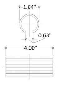
Item 08640 (70E-8) is an aluminum internal coupling (splice) that is designed to connect the ends of two equal pipes that are 1-1/2" IPS schedule 40 pipe in size.
