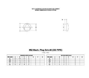
Machined aluminum end cap for schedule 40 pipe. See below for different pipe sizes that these end caps are avilable for.
