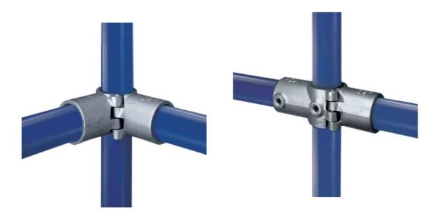
This fitting performs the same function as either KK21 or KK 26, but because of its unique "Hinge and Pin" system, it can be added to an existing tubular assembly. KKA21/A26 fittings are supplied and priced as a kit including 2 castings and 2 taper pins, which can be assembled in either configuration.
