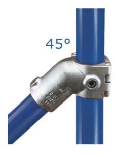
The unique "Hinge and Pin" system of this fitting enables existing structures to be easily extended without the need for dismantling. This fitting is most frequently used for bracing and struts.
