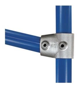
Used to join the middle rail to an end upright on a guardrail on a slope from 0° to 11°. Pipe cannot be joined within this fitting.
