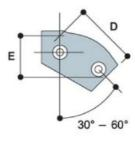
Designed as an alternative to the KK12 fitting, this adjustable fitting is most frequently used for bracing and struts. It may be used at any selected angle between 30° and 60°. As an alternative, it is possible to use KK29 in its vertical position in place of the KK27, using the KK27 only where a join in the pipe occurs.
