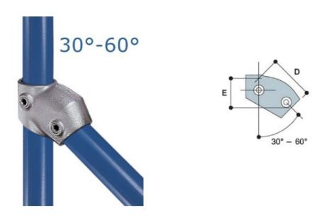
Designed as an alternative to the KK12 fitting, this adjustable fitting is most frequently used for bracing and struts. It may be used at any selected angle between 30° and 60°. As an alternative, it is possible to use KK29 in its vertical position in place of the KK27, using the KK27 only where a join in the pipe occurs.
