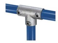
Most commonly used as the 90° joint between the top rail and an intermediate upright on safety railing. As there are two socket set screws in the sleeve, this fitting can be used where a join is required in the horizontal pipe. The KK10 fitting can be used as an alternative when a join in the pipe is not required.
