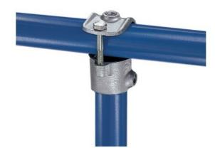
Widely used for adding to and modifying existing structures. This performs the same function as a KK10, but because of its open socket, it can be added to a complete structure. For alternative fitting, see KKA10. KK25 should be used when a join in the pipe is necessary.
