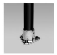
Item 27020 is made of aluminum-magnesium alloy 535.00 and includes two screws to hold the pipe in place. It is designed to hold 1" IPS pipe (see item A114ID).
