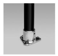
Item 26010 is made of aluminum-magnesium alloy 535.00 and includes two screws to hold the pipe in place. It is designed to hold 1" IPS pipe (see item A100ID).
