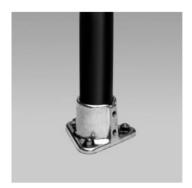
Item 25010 is made of aluminum-magnesium alloy 535.00 and includes two screws to hold the pipe in place. It is designed to hold 3/4" IPS pipe (see item A034ID).
