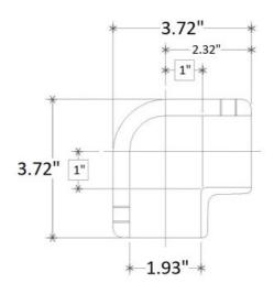
The Speed-Rail® 90 Degree Elbow is made of cast aluminum-magnesium alloy 535 and is available for pipe sizes 3/4", 1", 1-1/4", 1-1/2", and 2".
