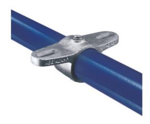
Designed for the secure fitting of various types of panels and flooring to pipe structures (i.e. plywood, plastic sheeting, wood planking, etc.) This fitting has two offset flanges to allow the flush attachment of panels to pipe.
