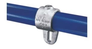
Designed for the securing of various types of panels and flooring to pipe structures. (i.e. plywood, plastic sheeting, wood planking etc.). This fitting has one offset flange to allow the flush attachment of panels to pipe. Often used with KKP51. See also KKP57.
