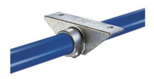
KK72 is a stair tread support suitable for most types of stair tread, including timber, open steel and checker plate. Fixing of the treads is by two bolt holes in each fitting. Ø indicates diameter of fixing holes. (Special Order Only) If KK72 fittings are to be used for a permanent application or subjected to high loads, the stair tread support pipe which is located at its ends with a single set screw, should be drilled and pinned to avoid rotational slip.
