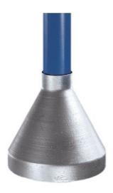
KK71 is a weather cap designed for roof guardrailing to ensure a weathertight seal for base fixing flanges. The weather cap is secured to the upright by means of a combined sealant and adhesive.
