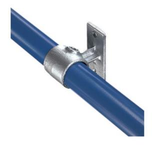
This fitting, with holes provided for countersunk flat head screw fixings only, is designed to carry handrails along walls or to fix structures back to walls. The pipe passes through the fitting and cannot be joined within the fitting. KK70 is also used to attach toeboards to the base of guardrail uprights. Ø indicates diameter of fixing holes. These fittings are not to be used as base flanges for full height guardrails.
