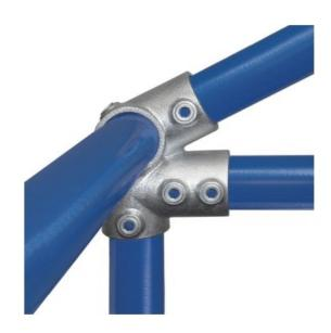
The Type 350 fitting has been designed for small structural building applications and provides for significant load rating. When used with the Type 351 ridge fitting a truss arrangement for additional support can be achieved. Double set screws are provided on the truss outlet to provide additional pull out resistance to hold structures firmly together.
