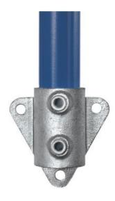
Side fixing for guardrailing and balustrading to walls, parapets, steps and ramps. The upright cannot drop through the socket.  $\emptyset$  indicates diameter of fixing holes. If the upright is required to pass through the fitting by machining out the base stop, the bottom fixing hole will be unusable.
