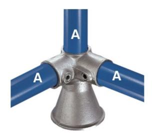
This fitting has been designed for the construction of post pallets. Incorporates sockets for the upright and side pipes, and a locating bell for stacking pallets. (Special Order Only)
