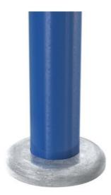
The Cover Flange slips over uprights to finish below ground post installations. The fitting is secured to the upright pipe with a single recessed grub screw.
