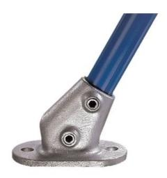
This fitting is similar to KK62, but is used to set up the upright at an angle between 45° to 60°. This fitting should only be subjected to light loads, which cannot be positioned at 90° to the applied load. For greater loads or other pipe sizes, a KK62 flange is used and the upright bent to the required angle. Ø indicates diameter of fixing holes.
