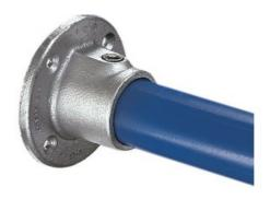
This flange, with holes provided for countersunk flat head screw fixings only, is used on structures where the fixing required is positional only. Frequently used as a wall fixing bracket. Ø indicates diameter of fixing holes It is not recommended for use as a base flange to support guardrailing or balustrading.
