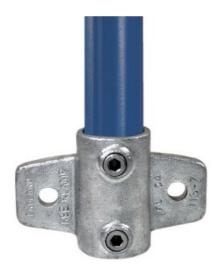
An internal swivel fitting, designed to accommodate varying angles on handrailing for staircases, ramps, or bracing. Used in conjunction with KK10, KK15, KK25 or KK45, it eliminates the need for specially drilled angle fitting KK27 and KK28.
