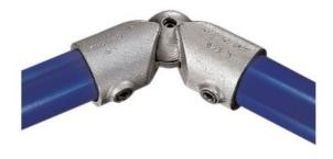
The KK53-8 fitting has been designed as a variable angle inline connection, adjustable through 202°. An entire structure should not be constructed from KK53-8 or any other swivel fitting, as these types would not provide sufficient stability or rigidity in the structure due to the free rotation of the fitting.
